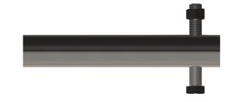
DIMENSIONS ARE IN INCHES TOLERANCES: FRACTIONAL±1/16 DRAWN HEATH 1/20/2012 RE-PN-1X601 PART # ANGULAR: MACH±1 BEND ± ASM # TWO PLACE DECIMAL ±010 THREE PLACE DECIMAL ±005 PIN,HINGE,MAIN, MATERIAL --
